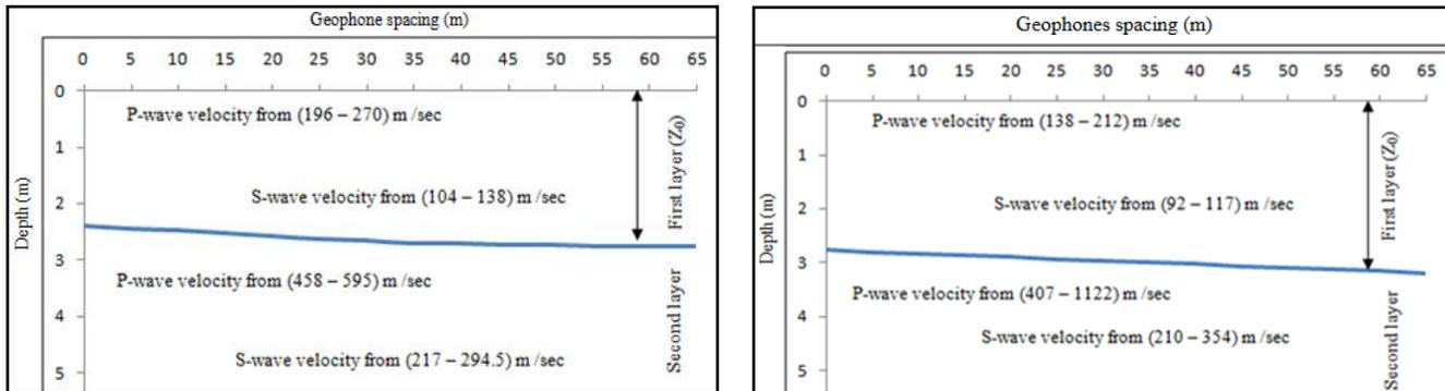
(Fig.10) Depth sections for Hilla-2 (left) and Karbala-2 (right)
