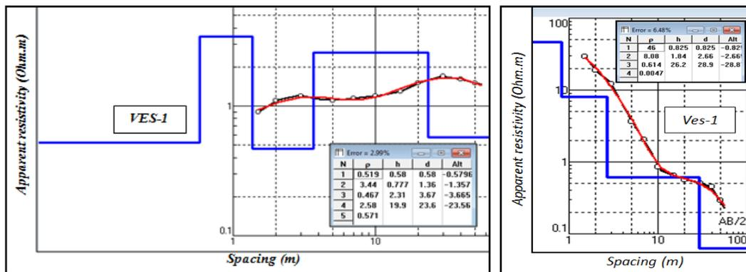
**Fig.3** Two examples of apparent resistivity field curves for Hilla-2 (left) and Karbala-2 (right) Plants
