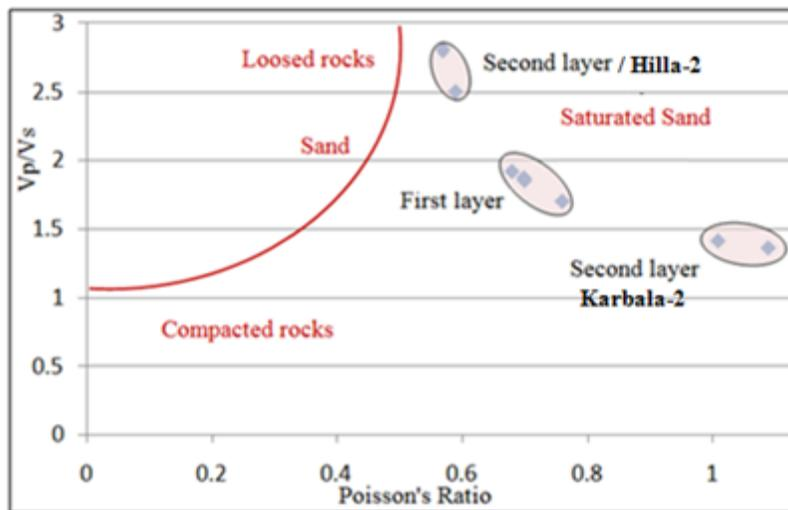
(Fig.13) Relationship between VP/Vs and Poisson's ratio for both Hilla-2 and Karbala-2 sites
