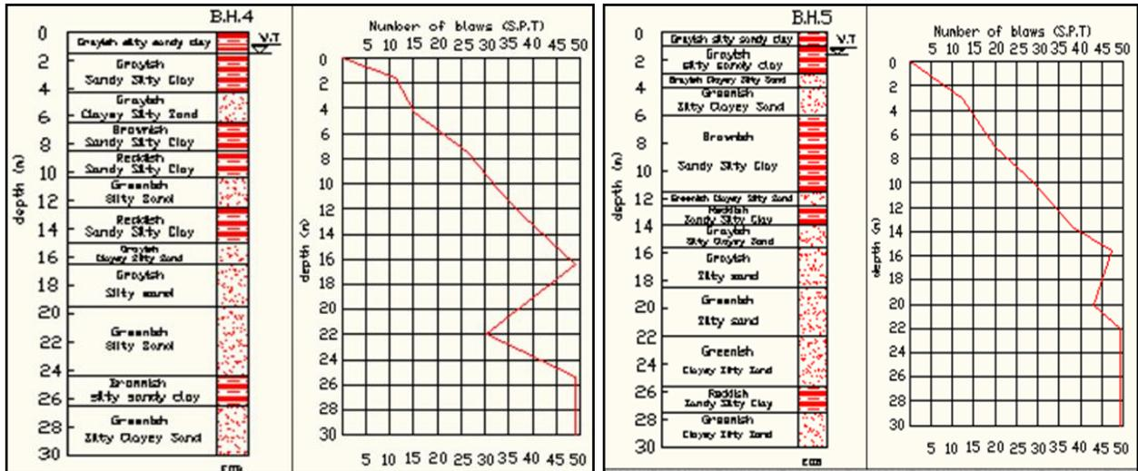
(Fig.11) Two examples of SPT for boreholes 4 and 5 inside Hilla-2 site
