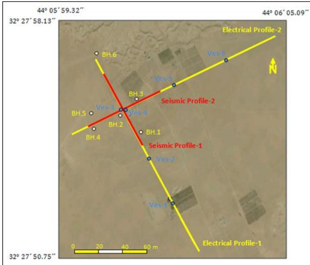
**Fig.2 Hilla-2 (above) and Karbala-2 (below) Plants showing profiles, VES and boreholes**
