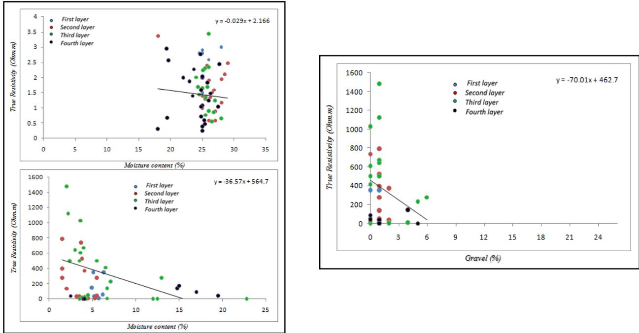
**Fig.6 True resistivity versus moisture content at Hilla-2 and Karbala-2 (left) and gravel at Karbala-2 Plant (right)**
