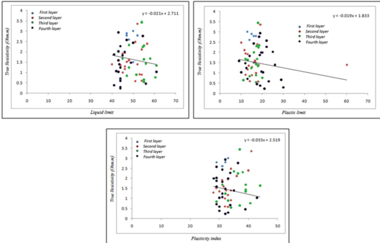
(Fig.9) True resistivity versus Atterberg (liquid and plastic limits and plasticity index at Hilla-2 and Karbala-2 subsurface soils
