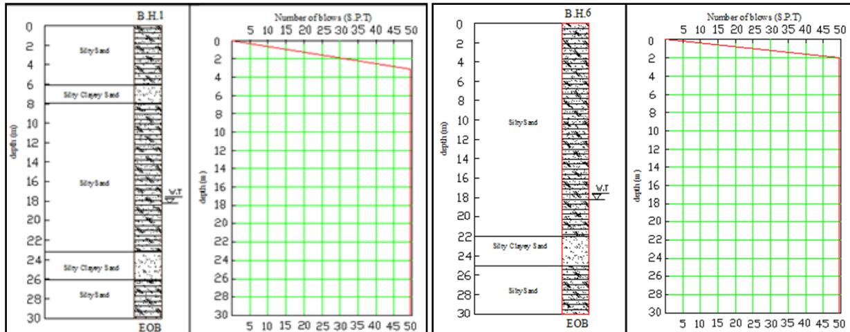
(Fig.12) Two examples of SPT for boreholes 1 and 6 inside Karbala-2 site
