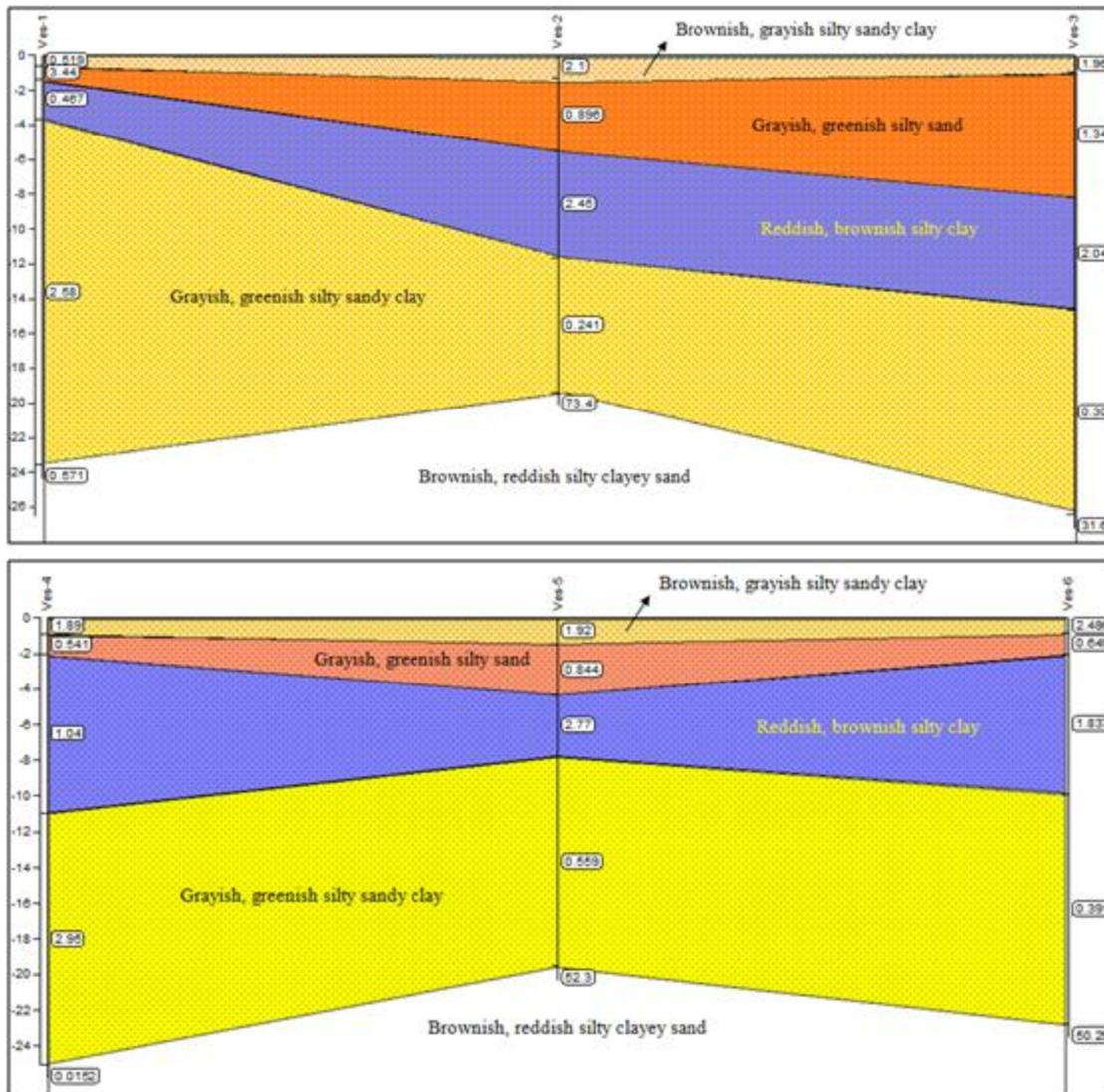
**Fig.4 Geoelectrical sections for profiles 1 and 2 inside Hilla-2 Plant**
