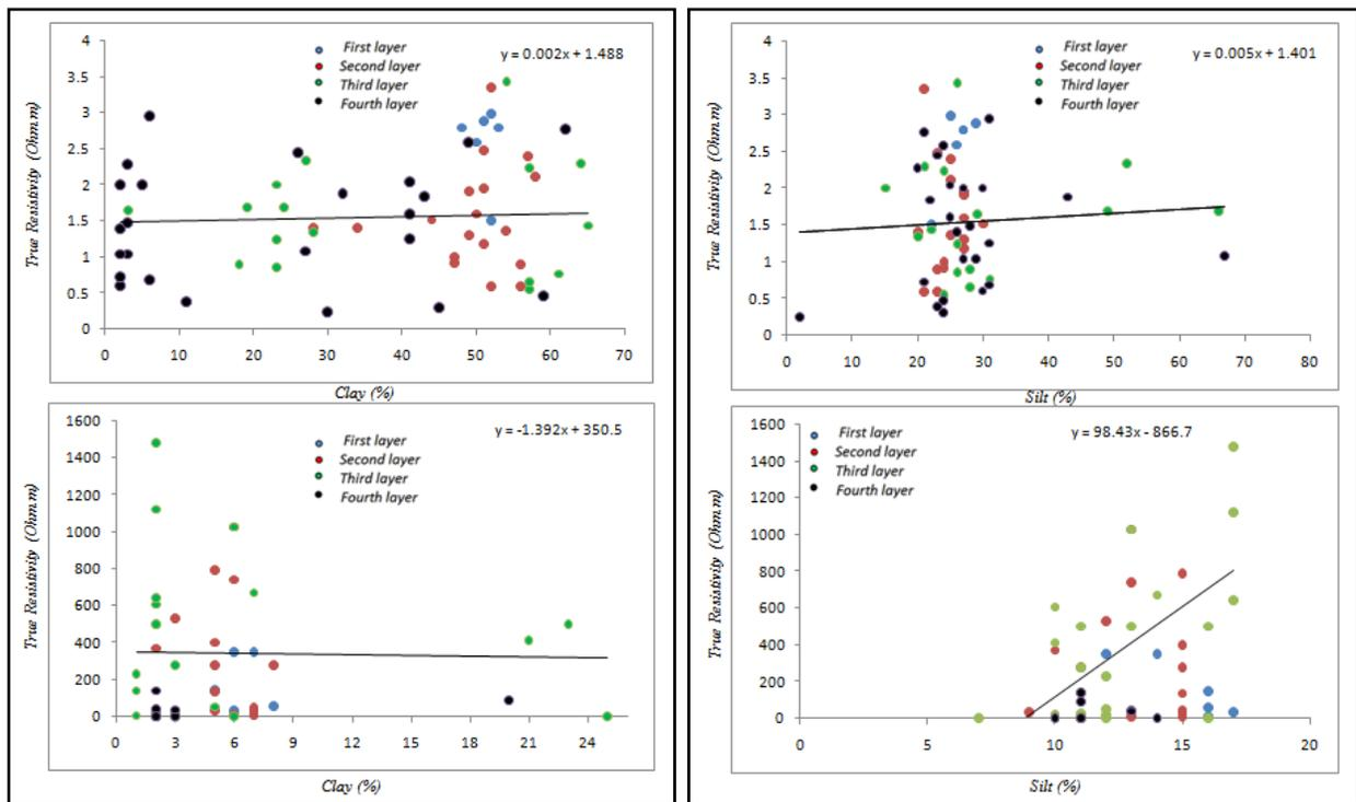
**Fig.7 True resistivity versus clay (left) and silt (right) contents at Hilla-2 and Karbala-2 Plants**
