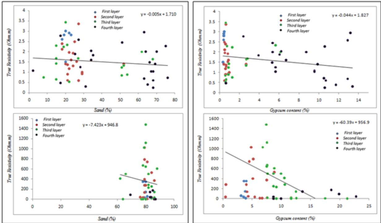
**Fig.8 True resistivity versus sand (left) and gypsum (right) contents at Hilla-2 and Karbala-2 Plants**
