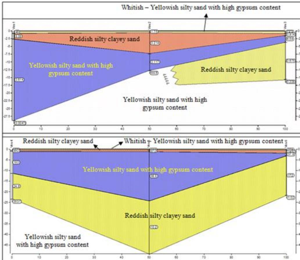
**Fig.5 Geoelectrical sections for profiles 1 and 2 inside Karbala-2 Plant**
